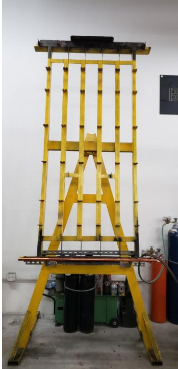
Figure 1. Original Braze Welding Jig
